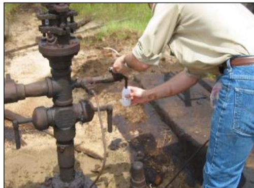
USGS Photo: Sampling produced water from an oil well in northern Louisiana.
