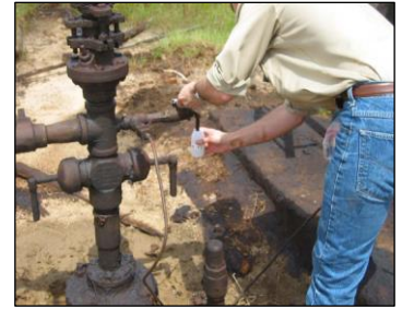
USGS Photo: Sampling produced water from an oil well in northern Louisiana.
