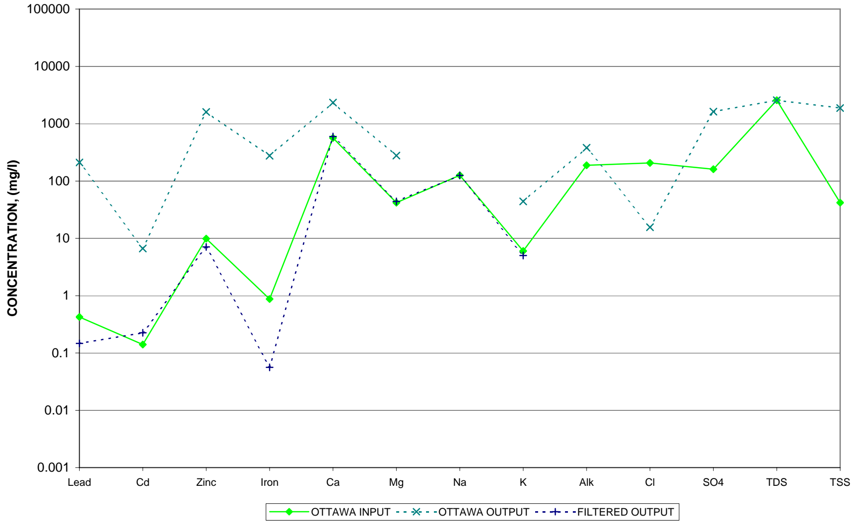
FIGURE 6: CHAT WASHING PROCESS WATER at the Ottawa Chat Pile
